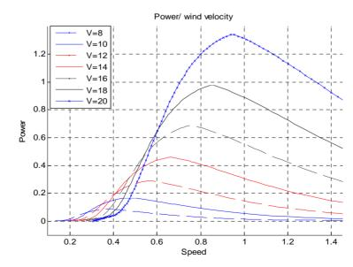
Figure 1. Output power in different wind speed with respect to  $\beta = 0^{\circ}$ .
