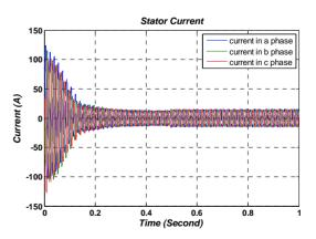
Figure 8. Stator current in DFIG in variable wind speed.
