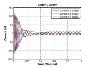
Figure 7. Regulated rotor current in DFIG in variable wind speed.
