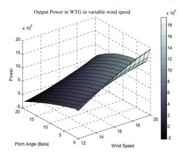
Figure 3. Output power of WTG in when speed of wind and pitch angle varies.
