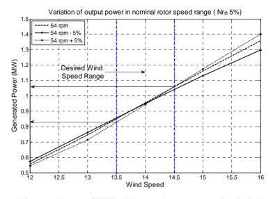
Figure 4. Generated power of WTG with constraint to rotor speed and wind speed.
