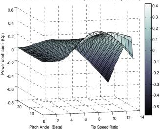
Power coefficient in WTG in variable wind speed and fixed rotor speed=54 r.p.m
