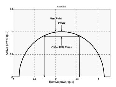
Figure 5. Active vs. reactive power generation curve in DFIGWTG.
