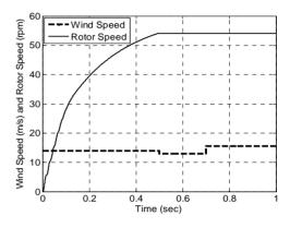
Figure 6. Rotor speed of DFIG in variable wind speed.
