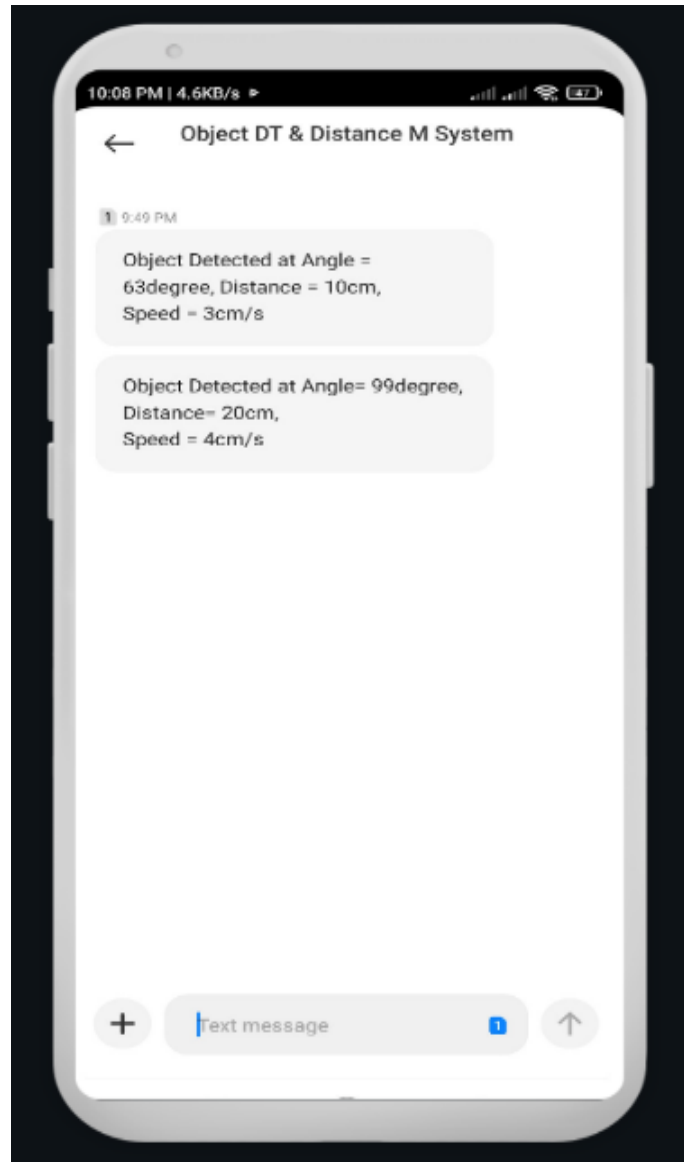
Fig. 12. Screenshot of object detection and distance measurement through SMS
