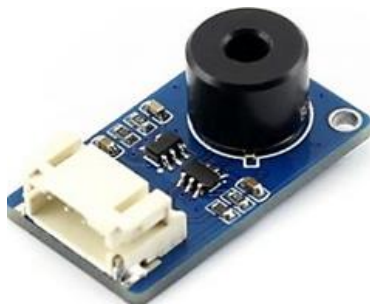
Fig. 3. Contactless infrared (IR) temperature sensor unit (Waveshare, 2023)
