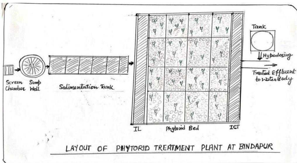
**Fig. 2. Structural elements of the phytorid treatment system at bindapur**
